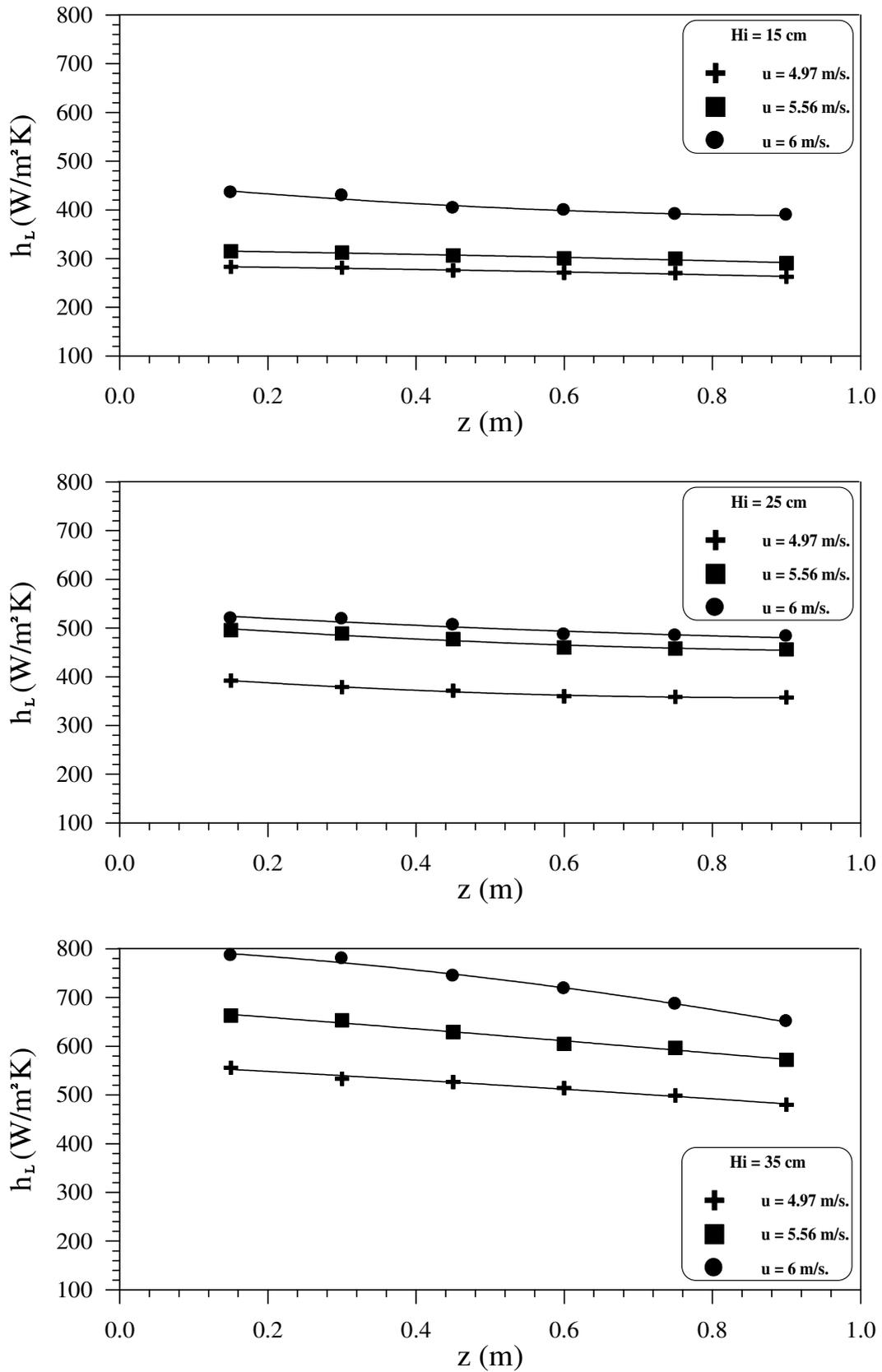
Figure (4): Local Heat transfer Coefficient Distribution.
