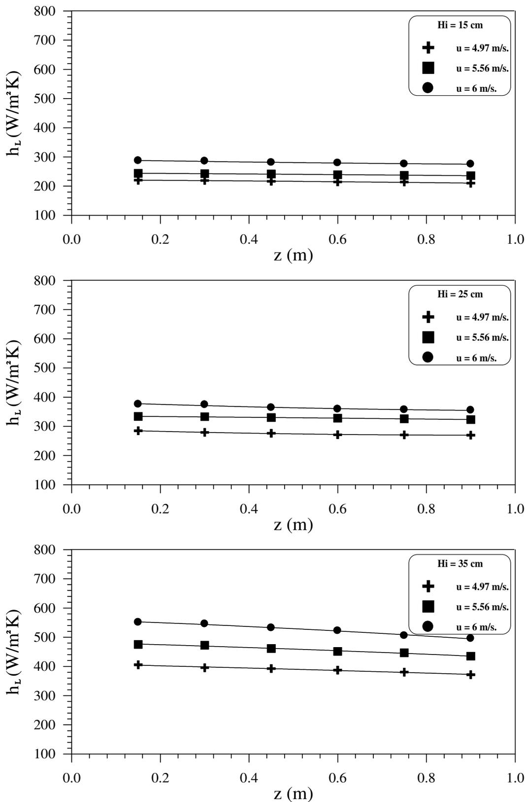
Figure (5): Local Heat transfer Coefficient Distribution.
