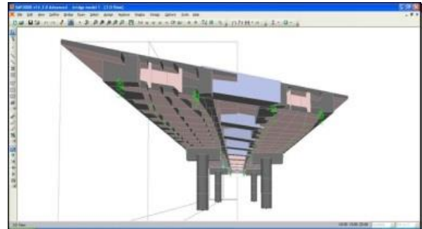
Figure 19. Web strengthening of box girder [43]
