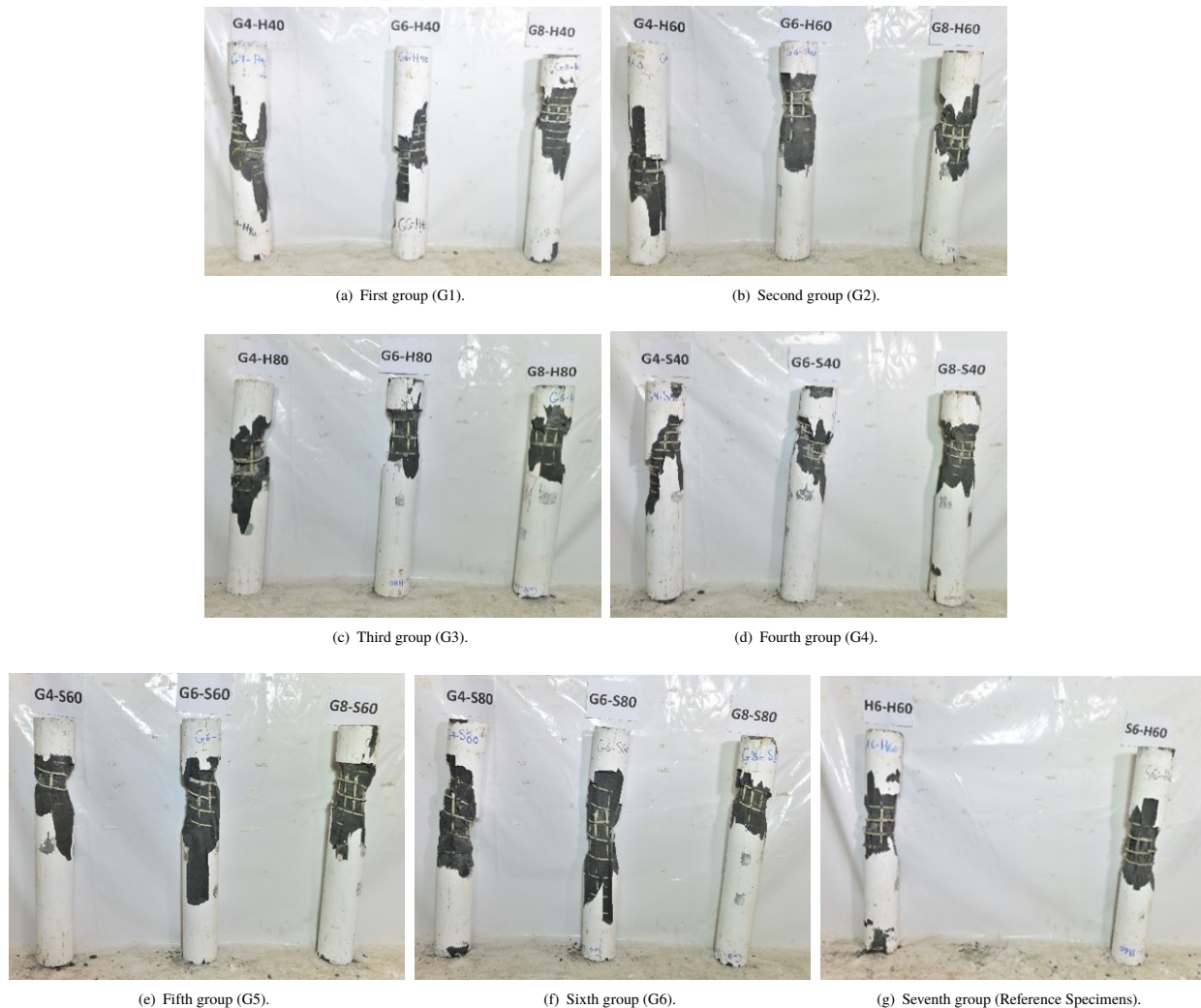
Figure 9. Failure mode of column specimens.
