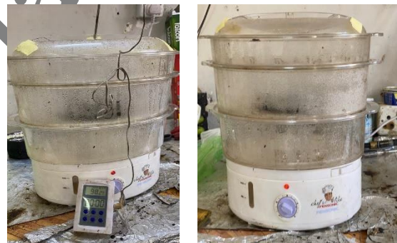
Figure 4. Steam Cooker Apparatus used in the aging process
