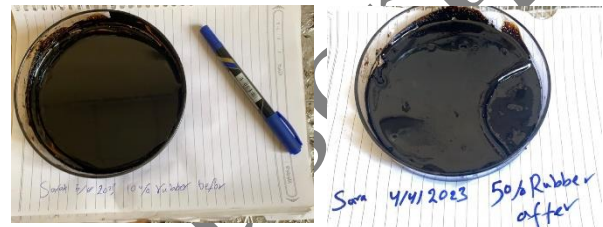
Figure 3. Asphalt Binders Before and After Steam Aging
