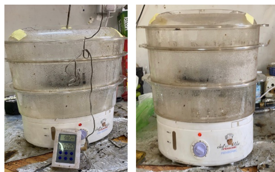
Figure 4. Steam cooker apparatus used in the aging process.
