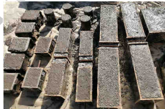
Figure 6. The wooden molds with the steel reinforcements.
