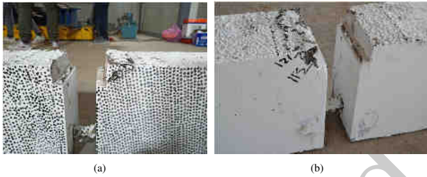
Figure 20. Flexural failure modes: (a) flexural rupture, (b) concrete crushing at the edges associated with rebar slipping.
