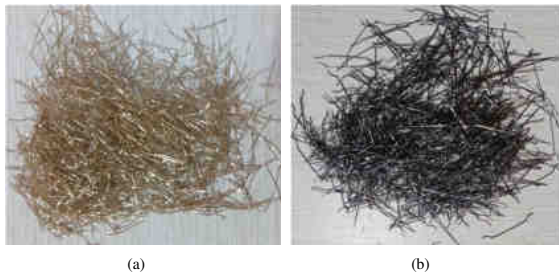
Figure 2. Steel fibres; (a) micro steel fibre, (b) hook end steel fibre.
