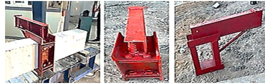
Figure 6. The steel lever arms used to generate torsional moment.
