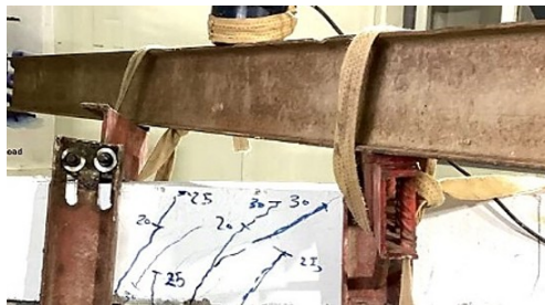
Figure 8. Failure mode and crack pattern of RB specimen.
