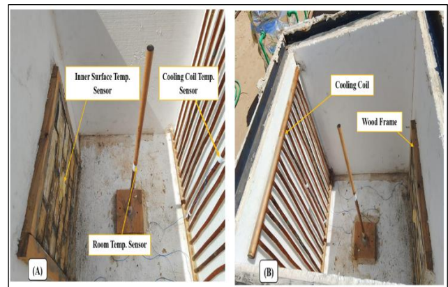
Figure 6. (A) and (B) represents the cooling system with thermocouple positions.
