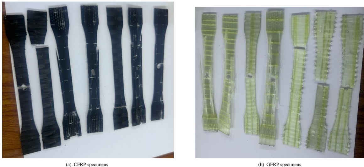
Figure 12. Comparison of fracture modes between CFRP and GFRP specimens under tensile loading.
