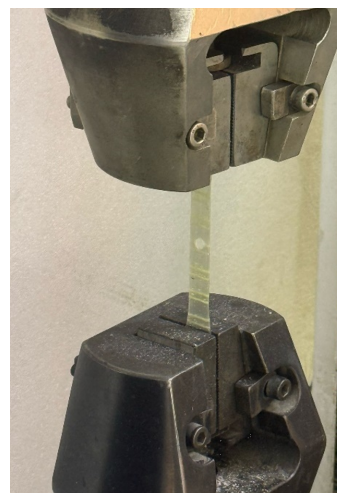
Figure 4. Typical tensile test of composite specimen.
