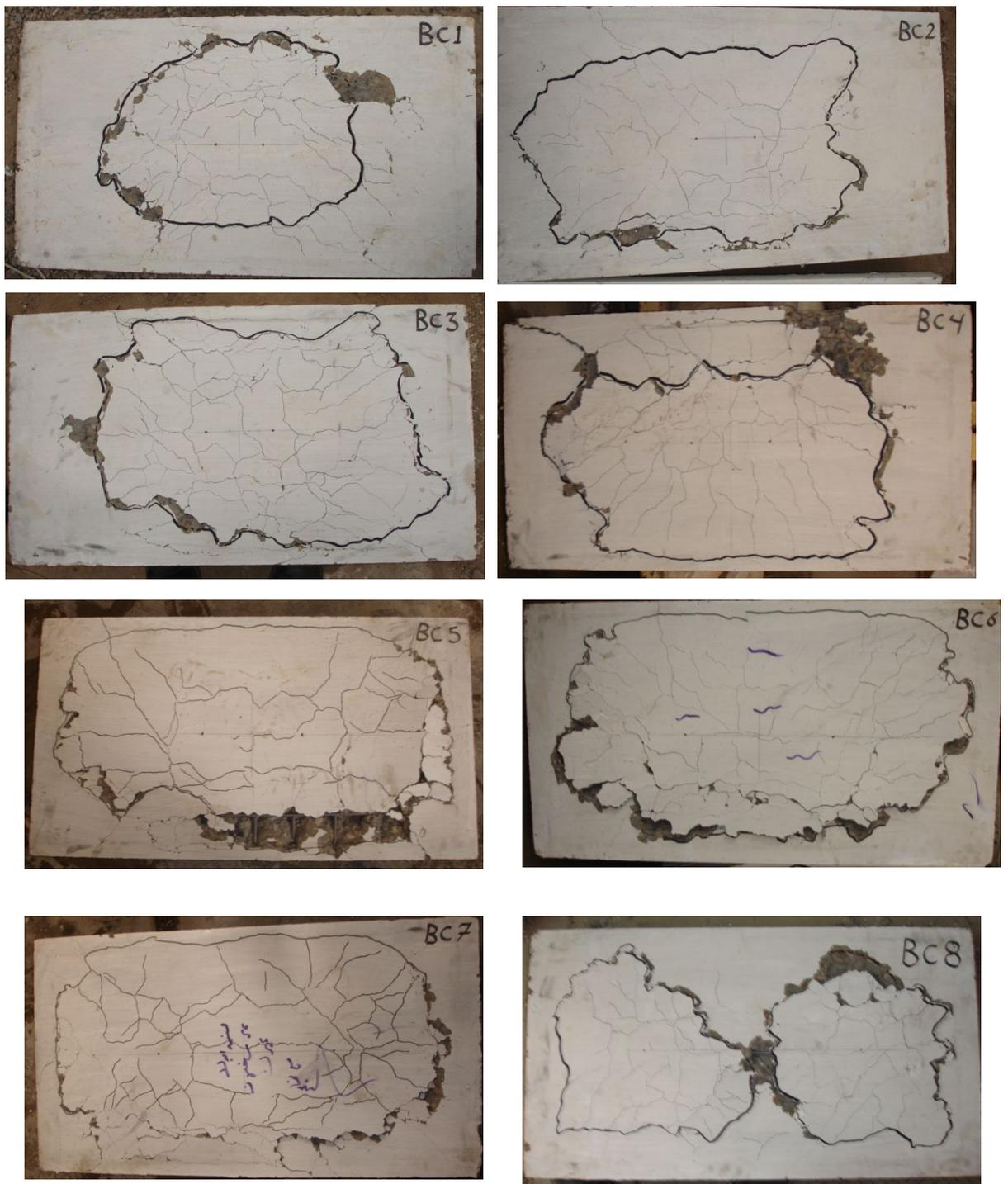
**Figure (4) Crack Patterns of Group (B) at bottom Face**
