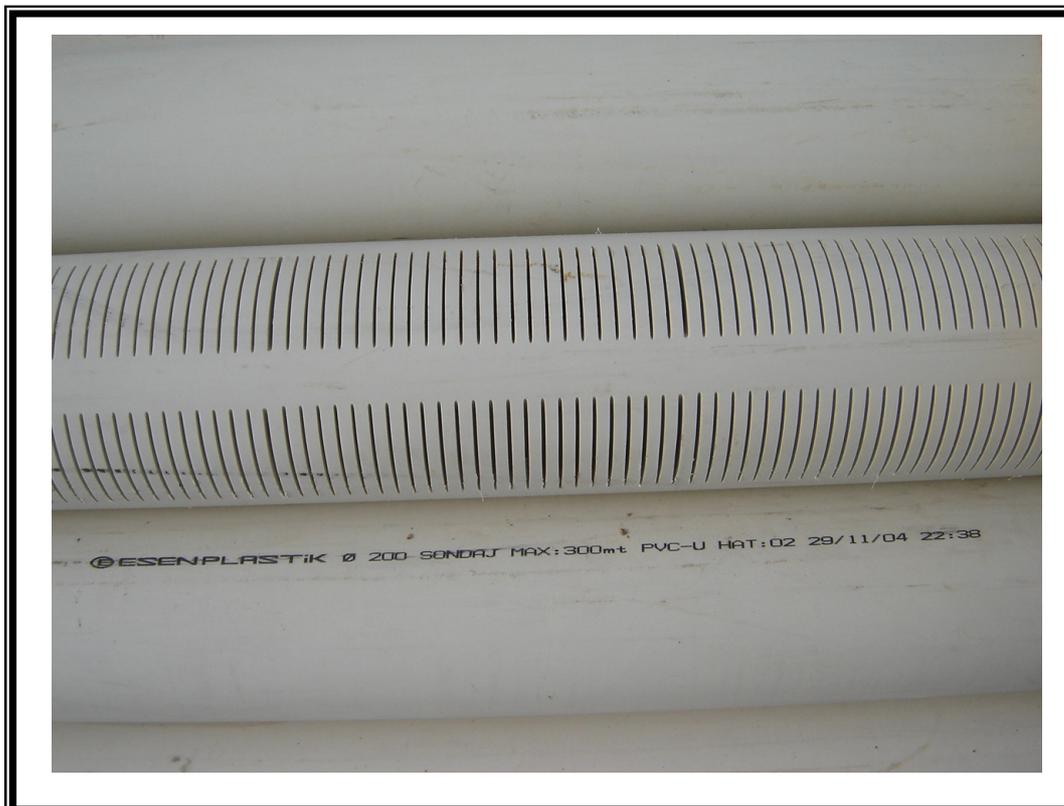
Figure (8) Screen filter pipes making in a special factory
