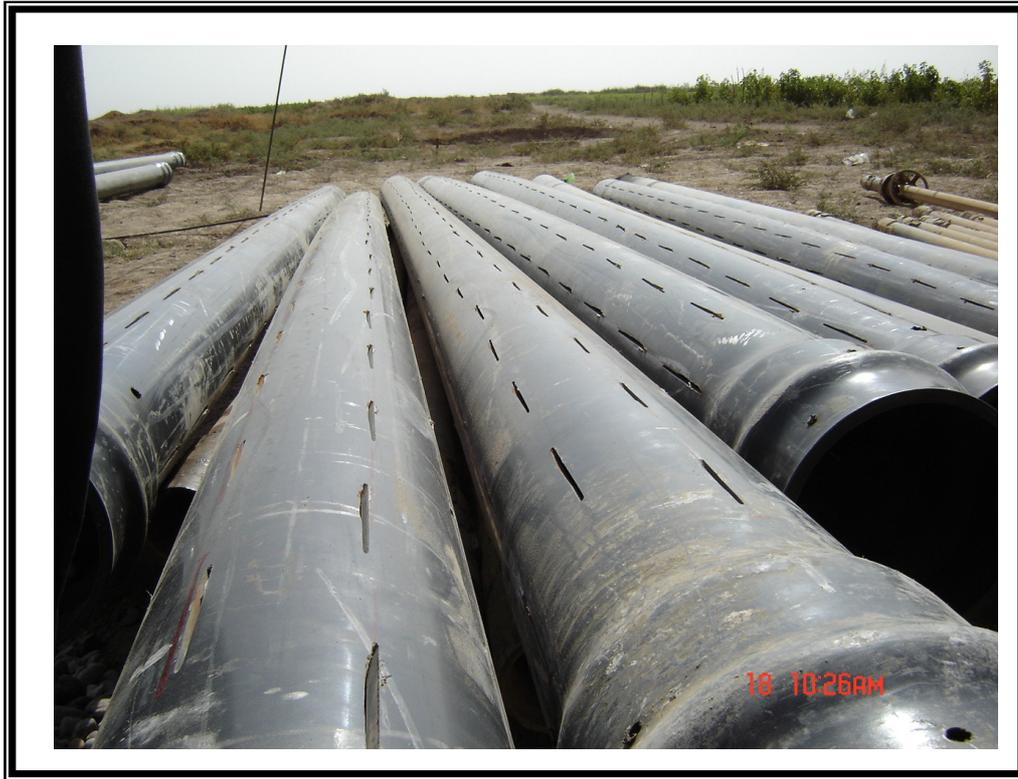
Figure (7) Screen filter pipes making in site
